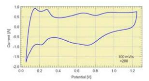
Cyclic voltammetry is based on linear voltage sweep between two fixed values.
