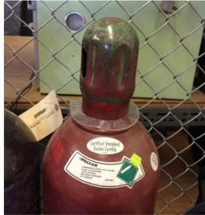
**Figure 9: Cylinder cap. Image courtesy of Safety Resources.**
